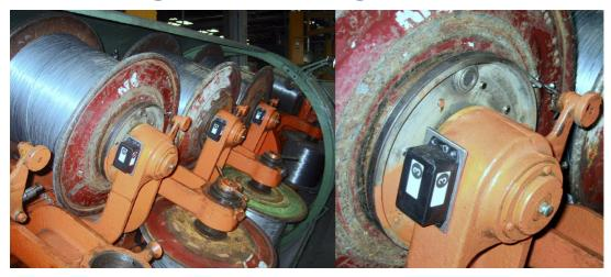
The usual wire break detectors based on the control of rotation of the reel can not be installed in machines having no sliding contacts brushes.
