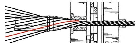
The wire breaks frequently in the cone of the forming die and often remains tight in that position, with the result that the break detectors based on the fall or on the count of wires do not work and the operator can not detect visually the break.
